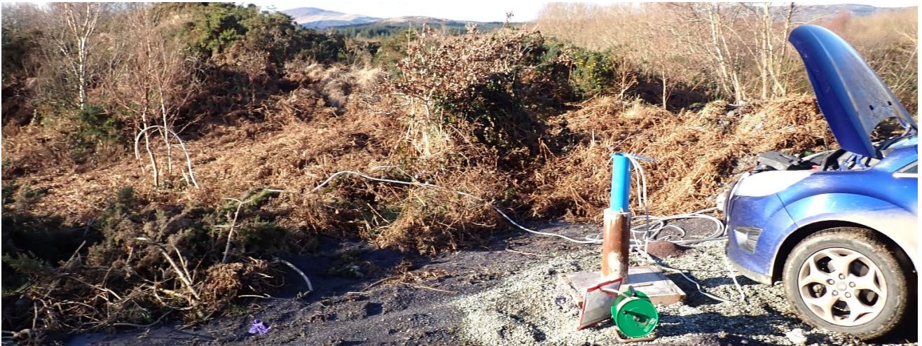
Photo 14: View of BH04 Headworks being pumped for sampling, (21 st January 2025).
