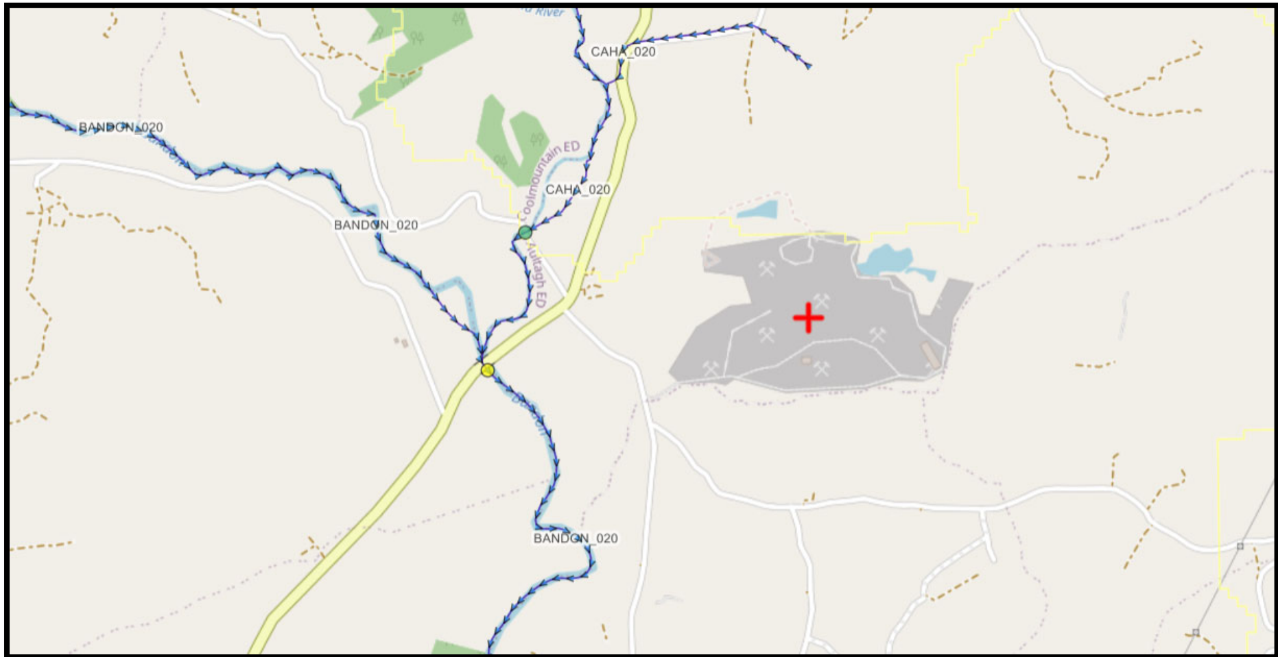
Appendix 7.1.2 – EPA Hydrology Mapping showing site location (red +), in the Bandon_020 River Sub Basin Catchment. (The north-western edge of the site is located along the boundary (yellow line) of the Caha_020 River Sub Basin Catchment.) The un-named stream that flows along the eastern and southern boundary of the quarry area is not mapped by the EPA. (Note that the course of the un-named stream is shown as a dotted line as it represents the local townland boundary.)
